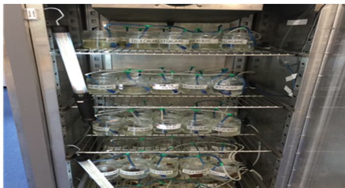
Figure 3 One of the experimental set-ups in the incubators showing the arrangement of the jars with one A. aquaticus in each jar exposed to experimental media (Solvent control (SCTR), Low treatment (LT) and High treatment (HT)).
